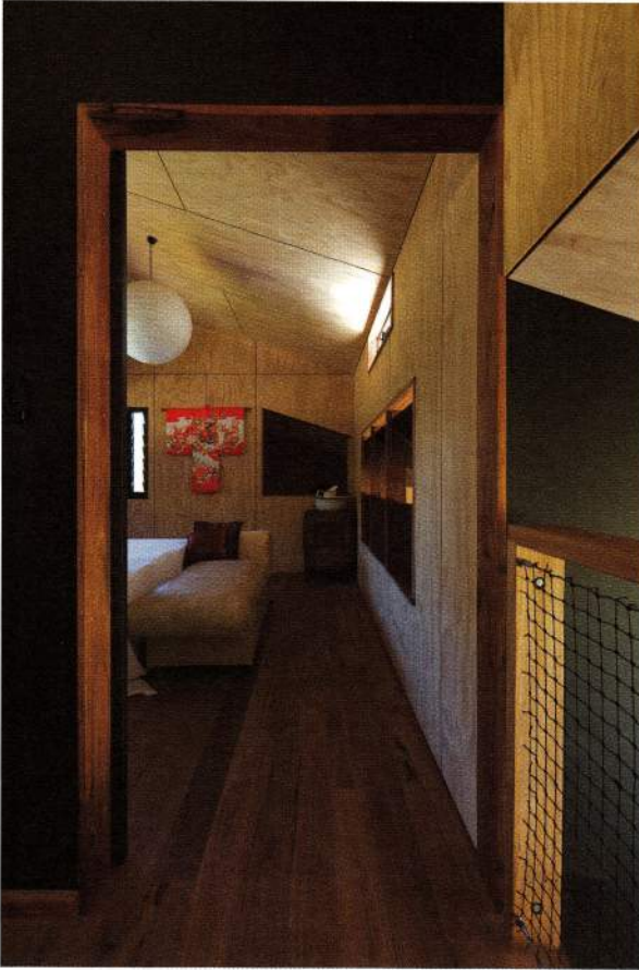
④ The loft bedroom looks out over the breezeway to the north. Walls are lined with locally milled Blackbutt and MDF.
