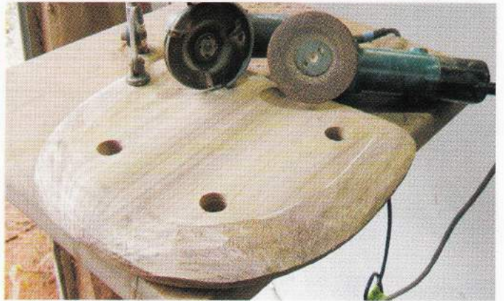
Photo.15: Contouring the underside of the seat
