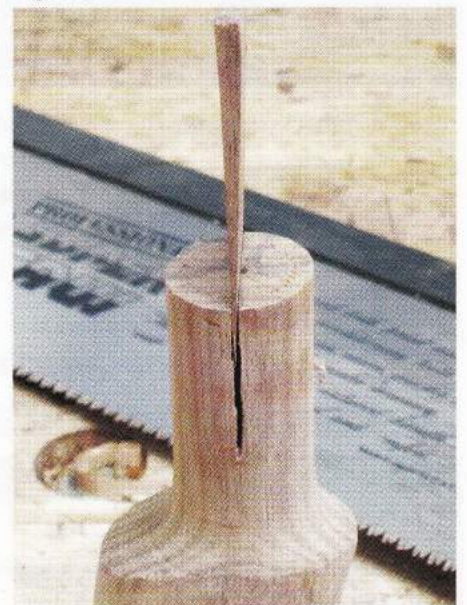
Photo.21: Checking the cut for the wedge in the top of the leg
