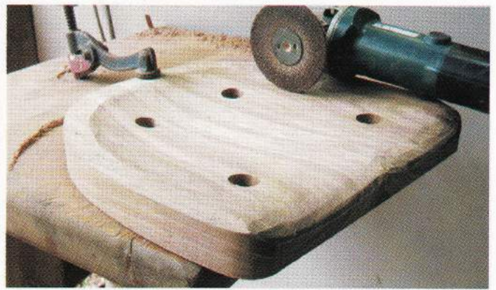
Photo.14: Refining the shape of the seat by sanding
