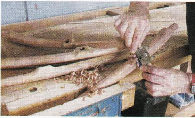
Photo.11: Using a spokeshave to refine the 'axe handle' shape of the top section
