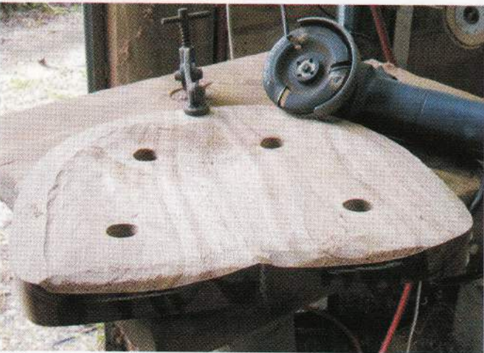
Photo.13: Initial shaping of the seat with the Arbortech TURBOPlane blade
