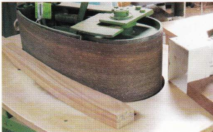
Photo.7: Sanding the inner curve on the legs back to the pencil line on the author's homemade linisher
