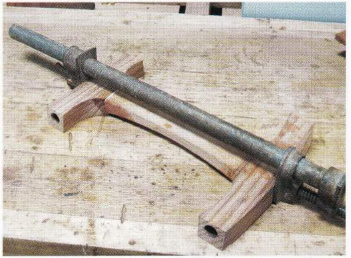
Photo.20: Rails and brace being glued together
