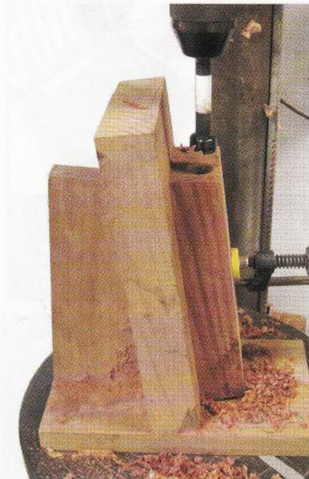
Photo.18: Drilling the dowel holes with an angled jig
