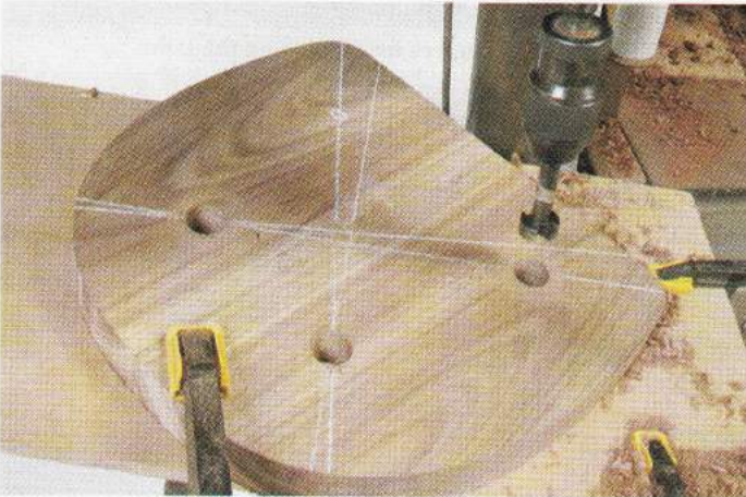
Photo.12: Drilling the leg holes
