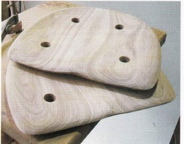
Photo.16: Two seats after final sanding with a random orbital sander, ready for the glue-up
