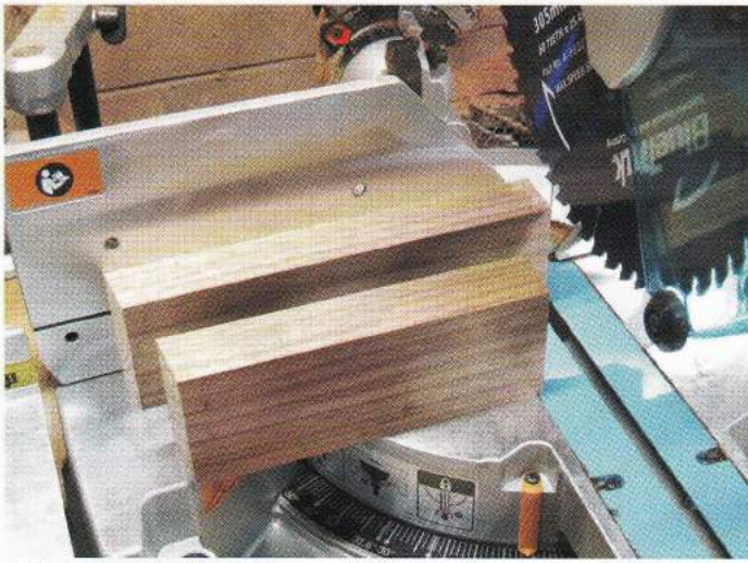
Photo.17: Cutting the 6° angle on the bottom rail
