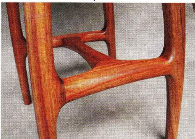
Photo.25: View of smoothed joints
